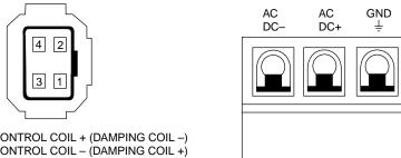
PIN 1 = CONTROL COIL + (DAMPING COIL -)
